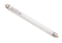
The device performs air sterilization with the sterilization effect of ultraviolet light. It destroys pathogenic microorganisms, viruses, bacteria, fungi and molds in the air. The lamp used in the device emits 254 nm of radiation. Hns 30w g13 bulb is used in the device. The device can work with 220 volts and 50 hz. ignition system is electronic ballast. 30w ultraviolet lamp is effective 20-25 m2 in 1 hour usage.
