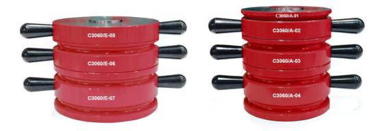
Distance pieces are used to reduce the amount of vertical clearance between the upper platen and the lower platen. 600 to 3000 kN machines are supplied with 205 mm and 165 mm dia distance piece.
