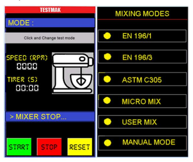
The mixer is started with the "START" button. The process steps defined in the mixing method are executed for the specified time. Mixer stops automatically when all steps are completed. When desired, it can be stopped with the "STOP" button. With the "RESET" button, the operation steps are reset and the process is returned to the beginning.
