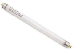
The device performs air sterilization with the sterilization effect of ultraviolet light. It destroys pathogenic microorganisms, viruses, bacteria, fungi and molds in the air. The lamp used in the device emits 254 nm of radiation. Hns 30w g13 bulb is used in the device. The device can work with 220 volts and 50 hz. ignition system is electronic ballast. 30w ultraviolet lamp is effective 20-25 m2 in 1 hour usage.
