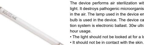
The device performs air sterilization with the sterilization effect of ultraviolet light. It destroys pathogenic microorganisms, viruses, bacteria, fungi and molds in the air. The lamp used in the device emits 254 nm of radiation. Hns 30w g13 bulb is used in the device. The device can work with 220 volts and 50 hz. ignition system is electronic ballast. 30w ultraviolet lamp is effective 20-25 m2 in 1
