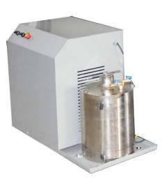
It is the cabin where the steam unit, electrical system and disinfectant tank fittings are located.
